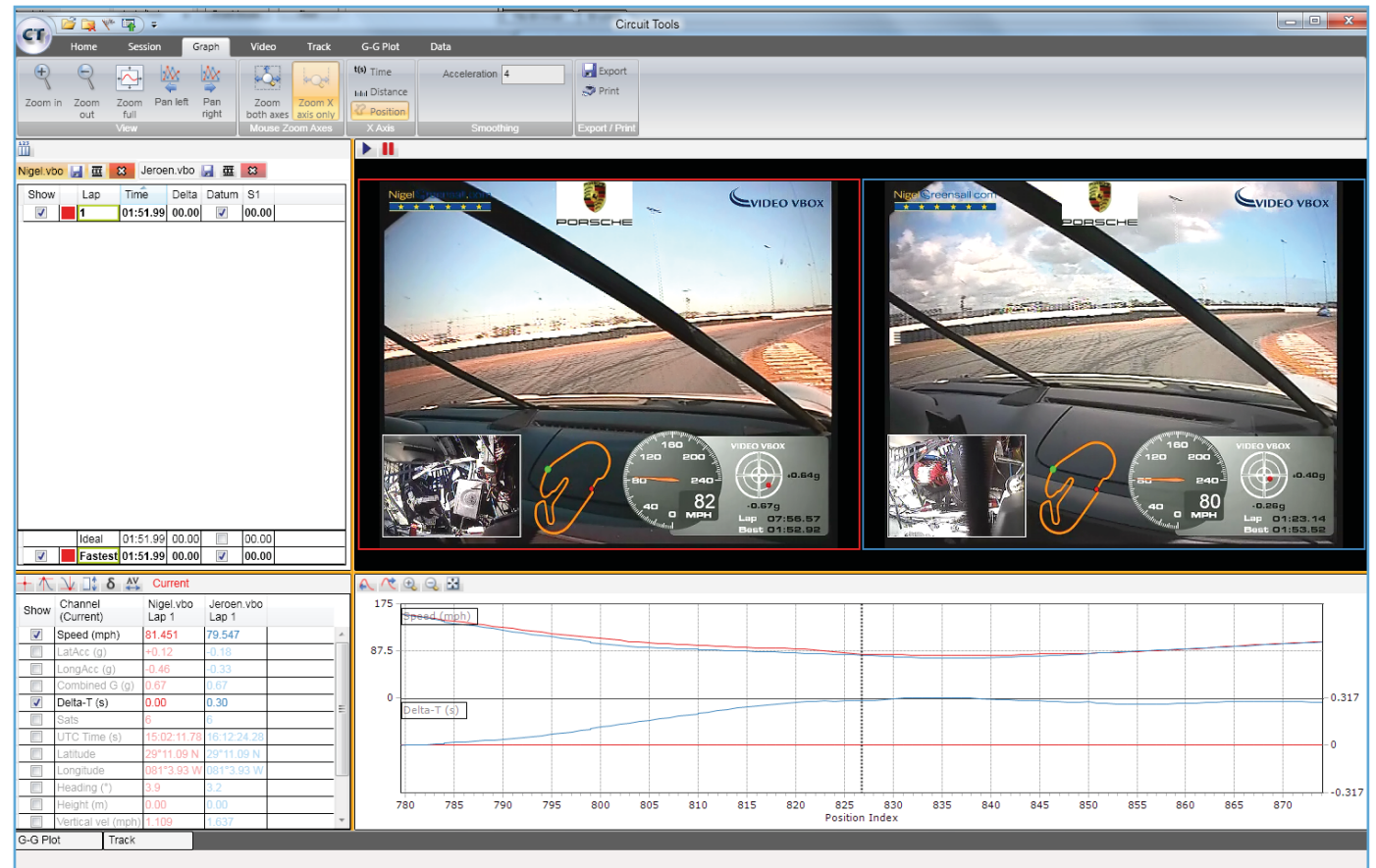
Figure 4 Apex of bus stop right-hander. We now have similar speeds, but look at the delta-t channel at the bottom: I have gained 0.3s in this short section
